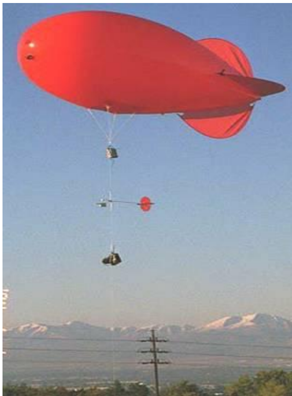
Figure 4: Tethersonde system by Vaisala carried by a blimp
